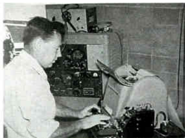
Bart Bartlett at his Model 26 teletype machine and Bohme CE keyer in the early fifties.
