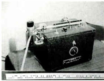
A siphon tape printer and sample tape, which reproduced the "undulations" of the incoming CW signal.
