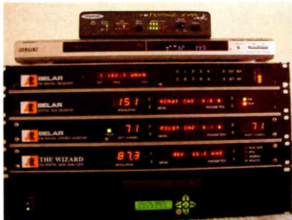
Typical test setup, including FMeXtra encoder at bottom.
