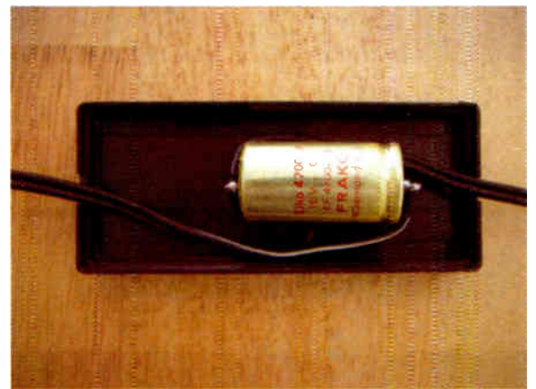
The capacitor fits inside the plastic box.
