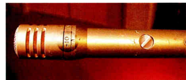
A Shure SM 81 with the 10 dB pad engaged.
