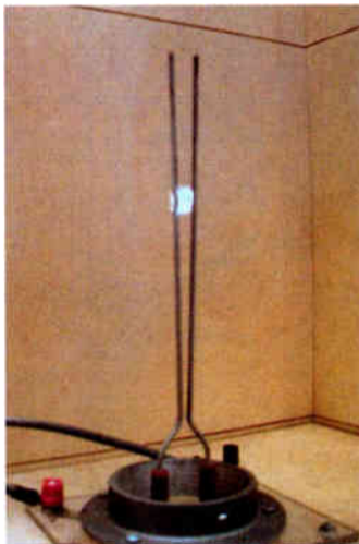
A Jacob's Ladder demonstrates lightning behavior.
