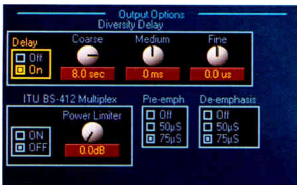
The diversity delay should be “on” and set to blend cleanly between digital and analog. Courtesy: Telos-Omnia
