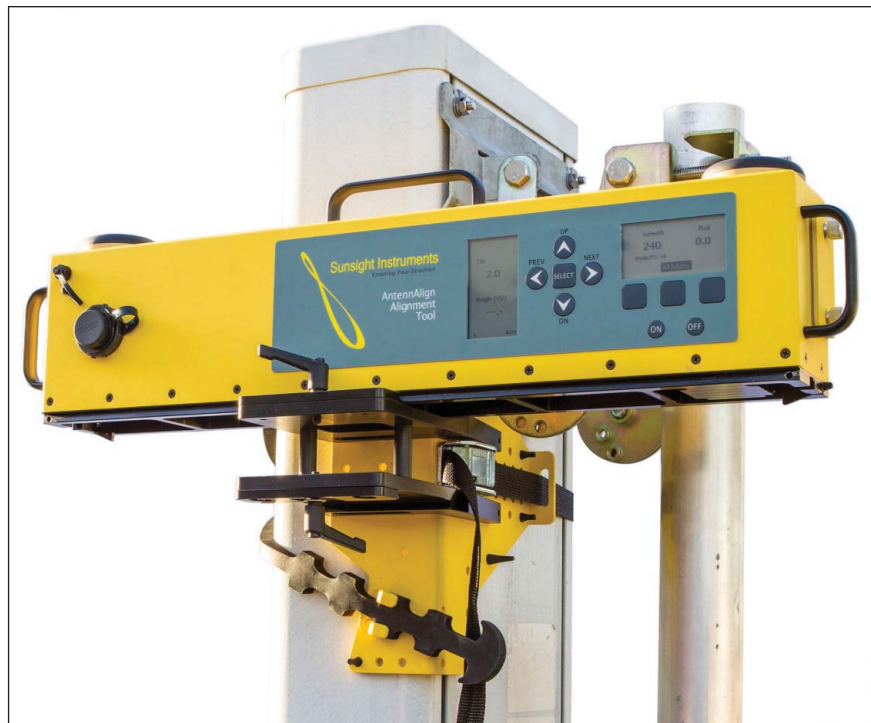
Photo 1. The AntennAlign alignment tool uses a unique design that integrates advanced accelerometers that allow it to capture downtilt and roll to the \pm 0.25 degrees mandated by carriers. It also incorporates a two-GPS system to produce real-time azimuth measurements of up to \pm 0.3 degrees RMS and \pm 1.0 degrees R99.
