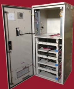
Site Support Enclosures CUBE SS Series supports VRLA or Ni-Cd batteries, various rectifier and power distribution options
