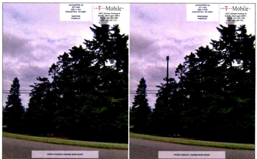
Photosim — View From H Avenue. To the left is the current view, looking toward the tower site from a vantage point on H Avenue, shown in the lower left of the aerial photograph. To the right is the same view with a simulation of how the 116-foot monopole with flush-mounted antennas would appear.
