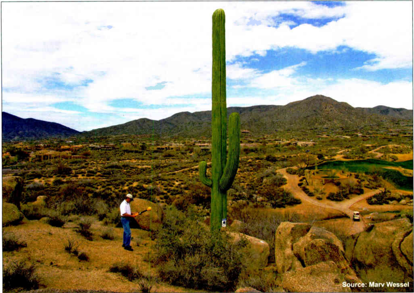
Marv Wessel is shown taking RF measurements near a cellular antenna disguised as a saguaro cactus. A person would have to scale the cactus to the antennas hidden near its top to receive unsafe RF exposure.
