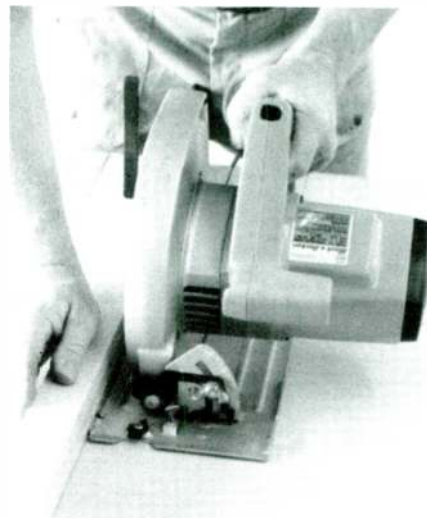
PHOTO 5: Using a straight board as a guide when cutting the stock. If you are cutting square pieces, the guide must be tested to establish that it is square.
