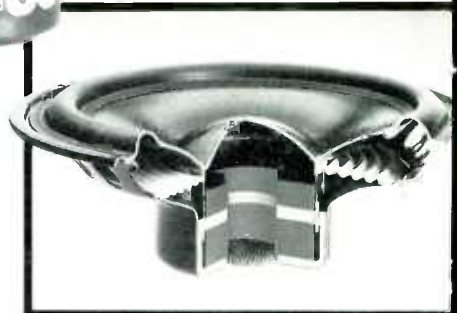
Typical Double Magnet Woofer Cross Section.
