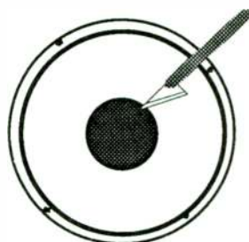
FIGURE 1a: Cut off dust cap.
