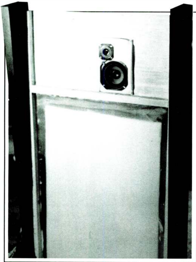
PHOTO 2: Mounted drivers on frame. Prototype used only a small anti-diffraction pad. Twin Mylar membranes, when shrunk, compress the foam diaphragm of the dipole woofer.
