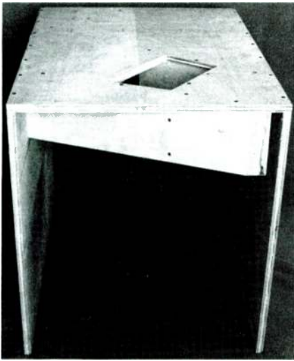
PHOTO 3: Positioning the top piece on the front and back panels.
