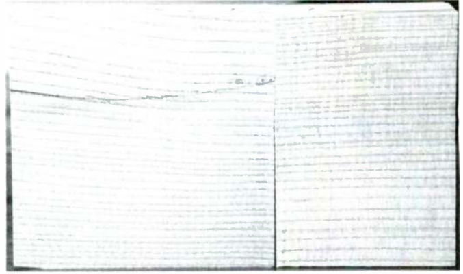
PHOTO 6: Saw blade check on a piece of 2 x 2 stock.
