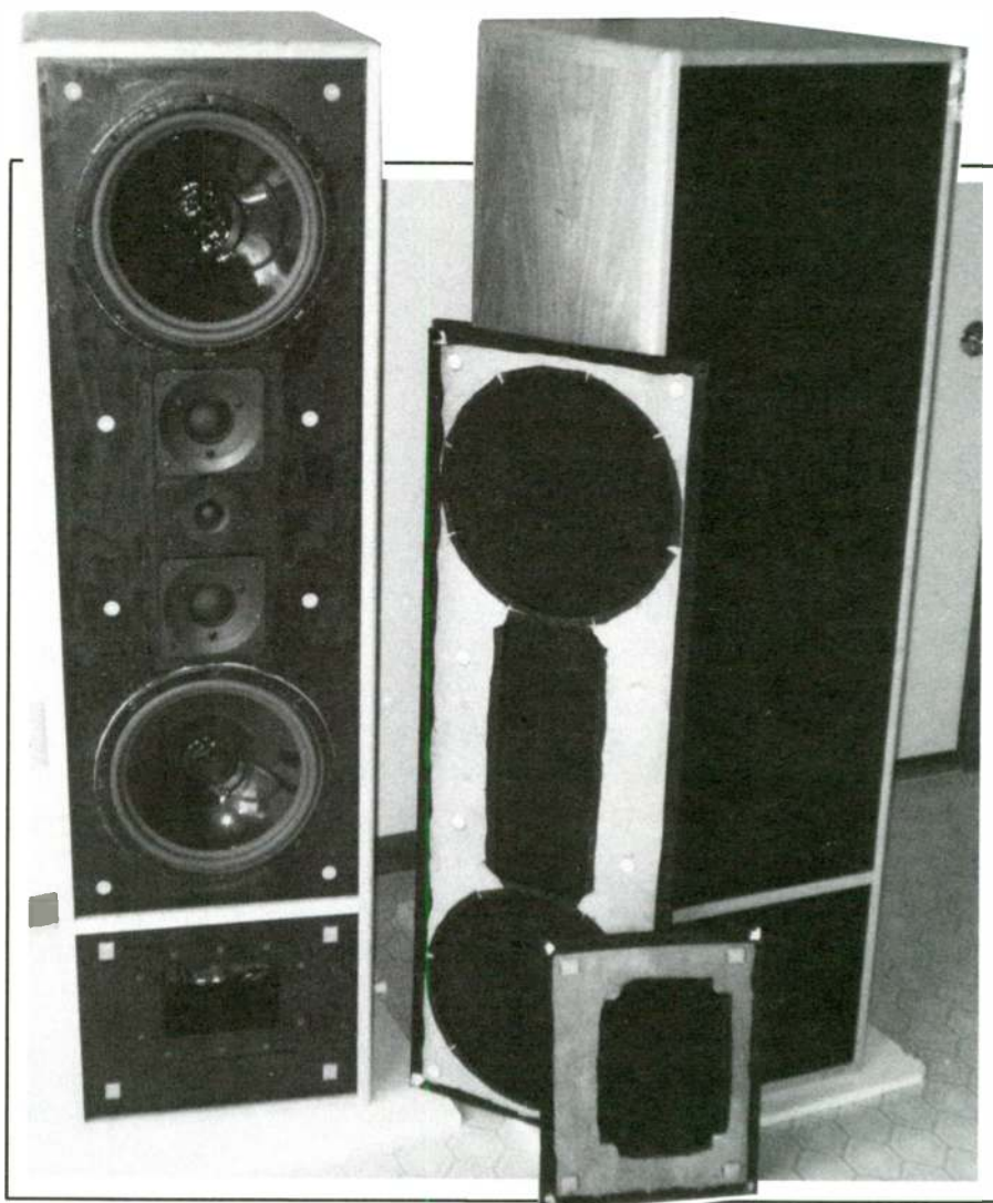
PHOTO 1: The finished speakers with the left channel grilles removed. Note the grille frame details and cone doping.
