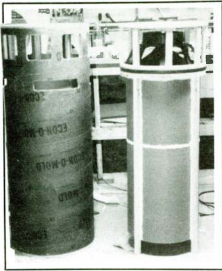
PHOTO 5: The outer shell and inner assembly. The speaker cradle, driver, and inner tube will eventually mount inside the outer tube.
