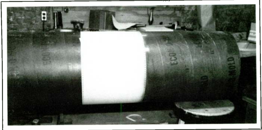
PHOTO 2: To cut the large diameter tubes squarely, use a piece of computer paper, spray paint, and a jigsaw.
