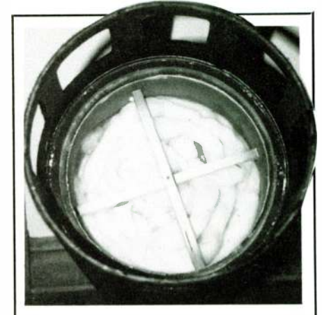
PHOTO 8: A top view of the cabinet with the driver and speaker cradles removed, showing the packing of the long fiber wool.
