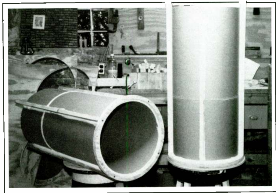
PHOTO 4: The inner tube assemblies, complete with pine spacers, ready for installation into the outer tubes.
