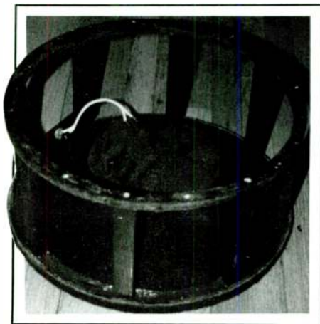
PHOTO 9: A completed revised speaker basket with the reflecting cone epoxied in place. The interior of the cone is stuffed with wool, and black grille cloth holds the wool inside the cone. Note the input jack and wire terminations for attachment to the woofer.
