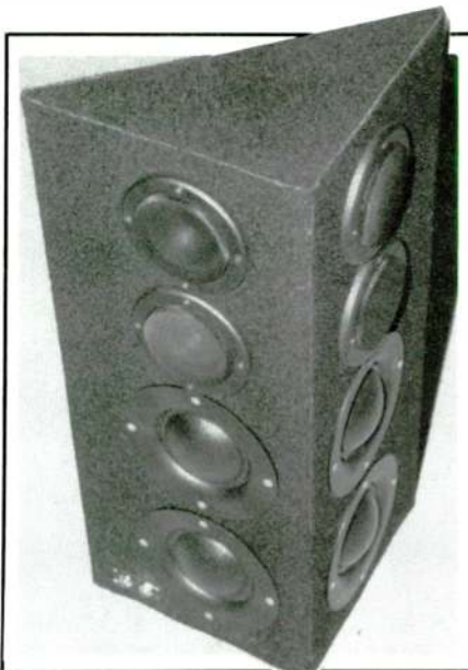
PHOTO 11: A completed tweeter cabinet.
