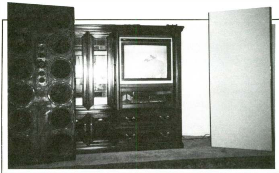
PHOTO 2: White grille cloth covers the driver array on the right unit of the pair. The dipoles flank a handsome equipment cabinet almost five feet high.
