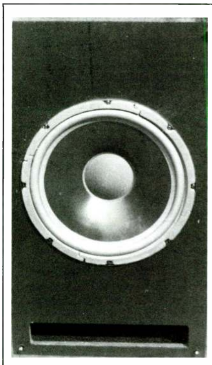
PHOTO 1: The VMPS smaller subwoofer, front view. The passive driver vents through the panel, at bottom.
