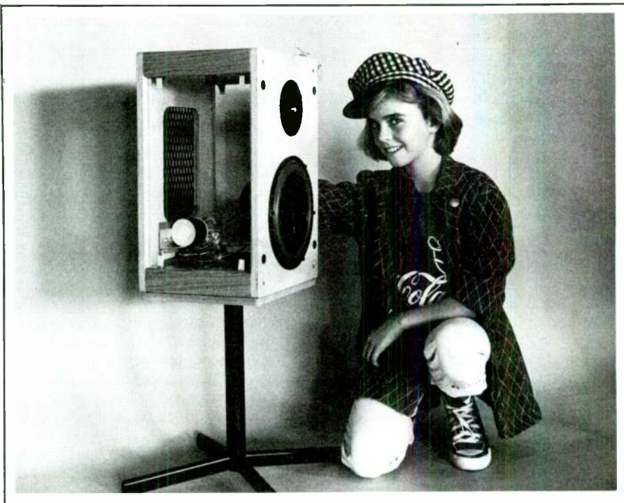
PHOTO 1: The nonrigid structure challenges conventional design enclosures.
