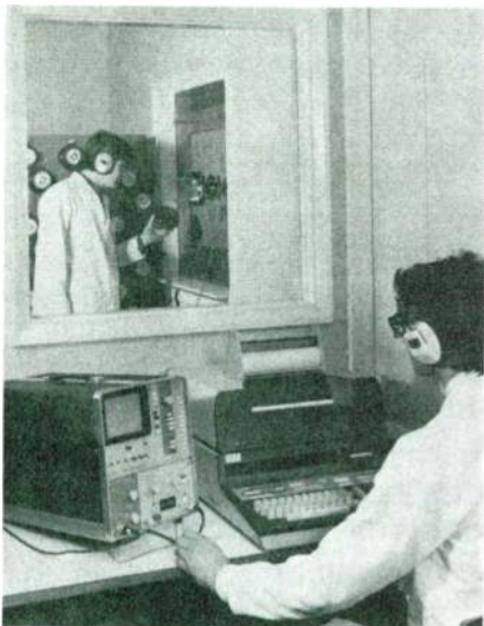
FIGURE 7: To find the proper mate for each drive unit, KEF uses impulse response techniques to measure each potential mate in a 94-unit batch.
