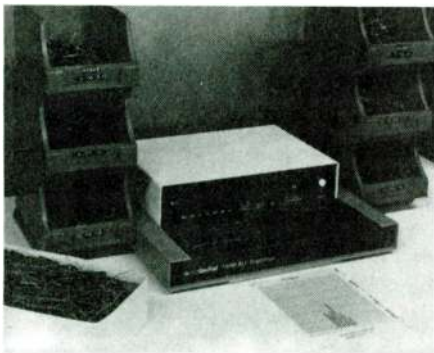
FIGURE 10A: Capacitors used in crossover networks are measured individually and sorted into 1 percent tolerance batches.
