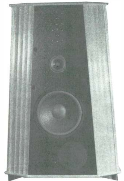
PHOTO 2: Otvos recently added black felt to the driver baffle, which is made of \frac{3}{4} -inch particle board and reinforced with heavy-duty plastic laminate.
