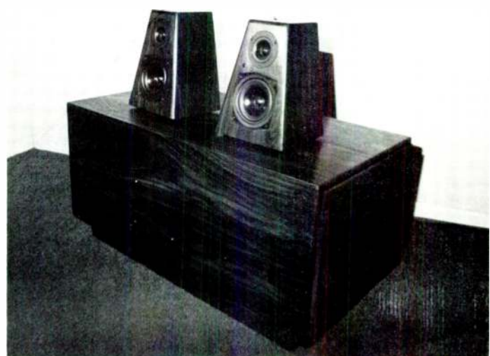
Photo B. Pyramidal shaped midrange tweeter cabinets include a 6.5" mid and 3" tweeter unit with crossover inside. Edges are rounded for least diffraction. The small enclosures are normally mounted as in Photo A.
