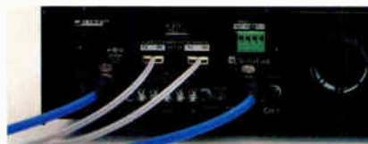
The plug-in QLink card is the EX amplifier interface, via fiber optic cable, to the MediaLink network. It allows for several optional I/O modules, including MMDI, PA-242, RS-485, and other glass or plastic fiber optics.
