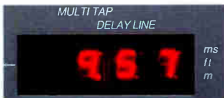
The display window provides information on the status of the IDL 1000. You can check or change the output delay times, delay units, and operation mode (stereo or mono).
