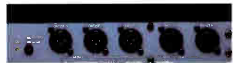
Two input and three output XLR connectors located on the back of the unit have corresponding level controls located behind the security panel in the front (transformers optional). An operation mode button sets the IDL 1000 to either stereo or mono operation. For extra protection against tampering, a lock switch is provided which makes the controls of the unit inoperative.
