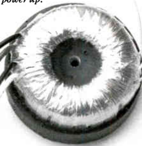
Torroidal transformer for greatly reduced AC hum.
