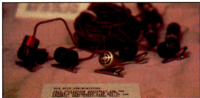
An assortment of RCA sub-miniature omni-directional mics, circa 1975.
