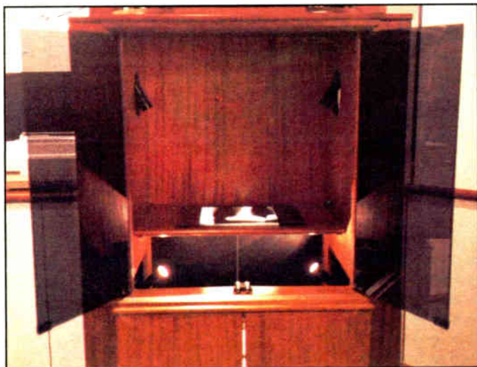
The graphics console is used to transfer art work, printed materials, sketches, overhead transparencies, or 35mm slides (or in this case, an x-ray) to video. An overhead camera is aimed down at the glass graphics table, which may be illuminated from the top or bottom.
