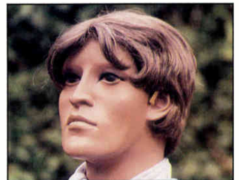
The author's homemade alternative to commercial binaural heads, with surface-mount microphone just visible at ear.
