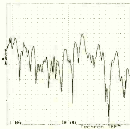
Figure 8 Frequency response 60 degrees "off axis," 0-20 kHz, 150 Hz resolution.
