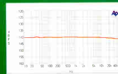
Figure 5: Digital I/O THD vs. frequency at 96 kHz and at digital full scale.
