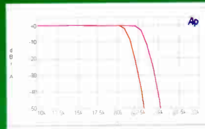
Figure 1: Frequency response at 44.1 kHz and 48 kHz.
