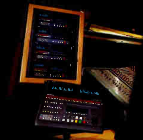
32-track M20 system with CADI™ Remote/Autolocator and RMD™ Meter Display at The Village, Studio D, West Los Angeles, CA
