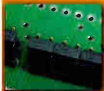
Jumpers behind each jack allows switching into 1 of 6 configurations, even after installation.
