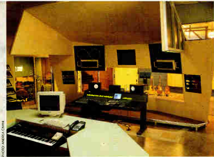
New production facility Studio 880 in Oakland, Calif., was designed by owner John Lucasey and includes two studios and a Foley stage. Studio A, pictured, is equipped with an 80-input Otari Concept 1 console (with moving fader automation and built-in dynamics), 5.1 monitoring including tri-amped active Genelec 1038As, Pro Tools 24, two Otari MTR-90II 24-tracks and a large collection of mics and outboard, both new and vintage. ▼
