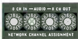
No computers for configuration or operation. Change routing at a turn of a switch.
