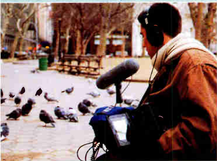
Ben Cheah recording sound effects with a Neumann 191i stereo mic in an MS configuration, onto a Sony Pro II DAT. He also is using an 8mm playback unit (in hand).
