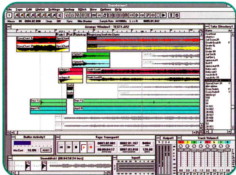
Figure 1: The Arrange window displays Parts, selected from the Take Directory. Track views can be expanded both horizontally and vertically.
