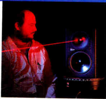
Mackie acoustic engineer David Bie uses scanning laser vibrometry to map HR824 tweeter dome vibrations. Film at 11.
