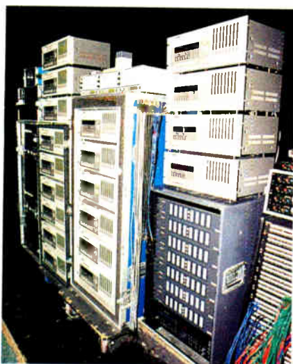
Left: the portable machine room of Tascam DA-88 record/playback units. Right: a bank of Lexicon LARCs, with a few of the predubs on DA-88 cassettes.
