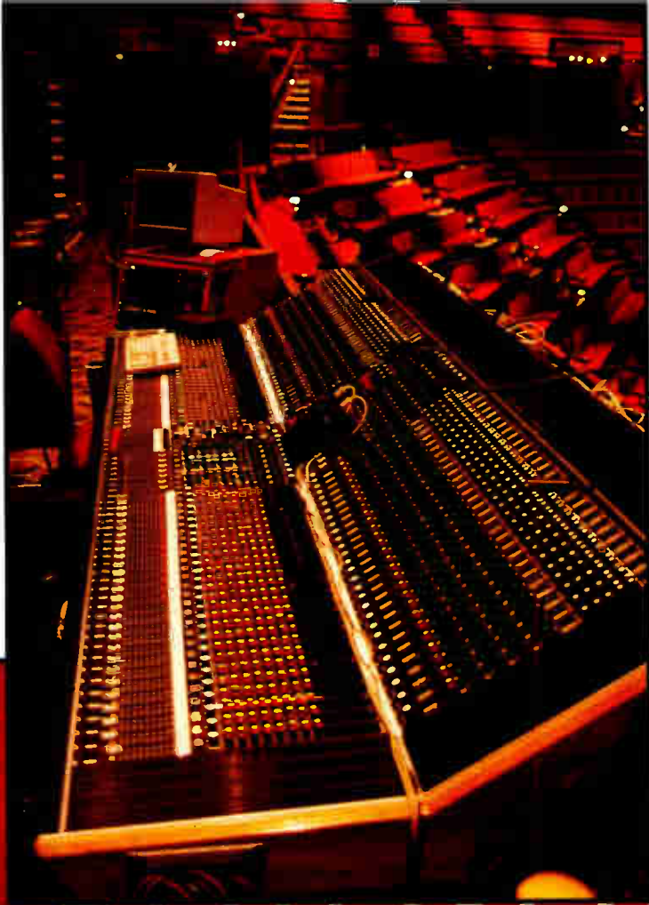
Above: viewing the stage from the house mixing position; left: the Paragon ATI 56-channel house console below: The Opry House in full swing
