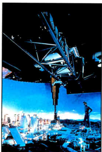
TCI's motion-control camera gantry system looms over one of the miniature sets for the "Theater of Time."
