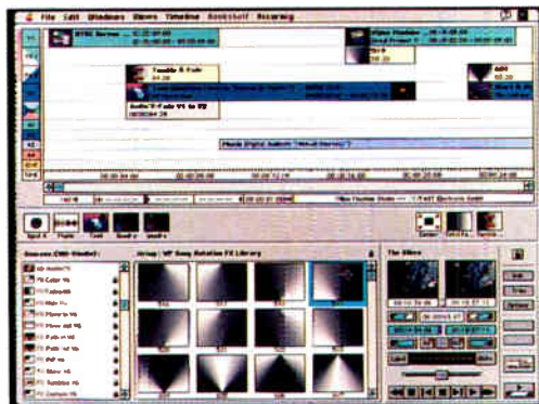
Fast's Video Machine Studio software is an edit controller that also allows the addition of effects, graphics and titles. (p. 91)
