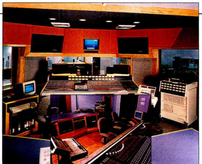
Equipment includes a DDA DMR-12 32-input console, an Otari MX-80B 24-track recorder and two Studer Editech Dyaxis digital audio workstations.
