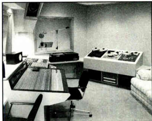
Above: TMP Recording, Berlin, N. J. Completed in August of 1990, TMP Recording was designed by owner Tom DiGangi. The facility offers a 32-input Tascam M3500 console, a MIDI studio and Tascam 16- and 24-track recorders.
