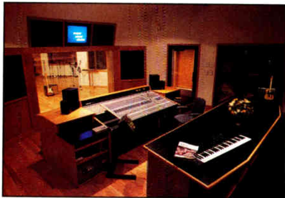
Left: Meyer Sound Studios, Bismarck, N.D. Designed by Bill Morrison of Acoustical Physics Labs, the control room uses sprayed wall geometry and a staggered wedge ceiling design to achieve a large reflection-free area. The facility opened in March 1991 and includes a Neotek Elite console and UREI 813 monitors.
