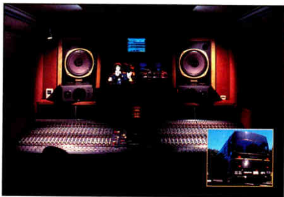
Above: Manhattan Center Studios remote bus, based in New York City. Housed inside a 40-ft. Prevost is a Neve VR48 with Flying Faders, two Sony PCM-3348 digital recorders and a Tannoy/Perreaux monitoring system. The bus, designed by Manhattan Center Studios staff with consultancy by Richard Rose of Hot House Professional Audio, hit the road in the spring of 1991.
