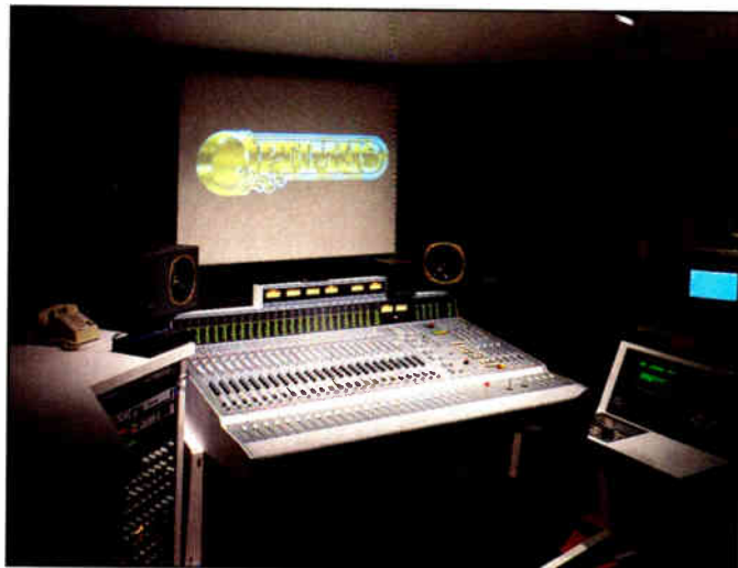
Above: Optimus, Chicago. This film and video mixing suite and post-production room is equipped for multichannel Dolby film mixing. Designed by Mark Sarantakos, the room was completed in the fall of 1990. The room features a Neotek console, an AMS AudioFile and Tannoy monitoring.
