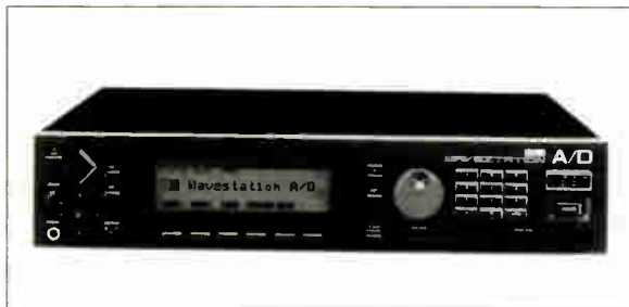
With an audio input, Korg's Wavestation Rack can be a synthesizer or signal processor.
