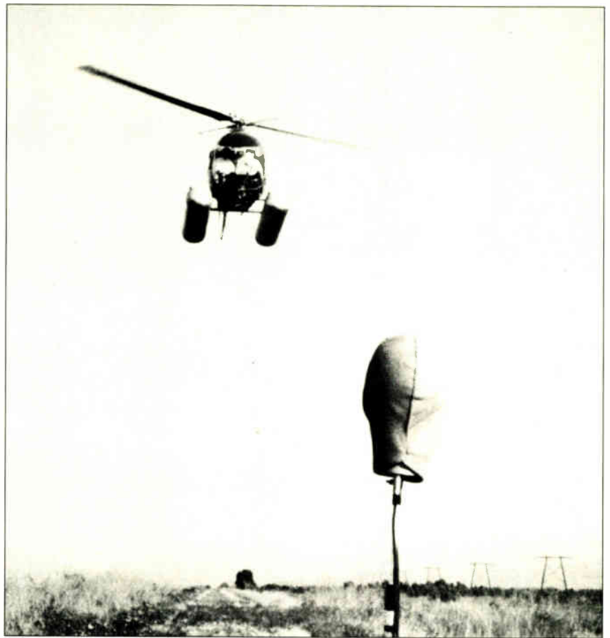
Holophonics system in use on location in the Florida Everglades, recording stereo sound effects of helicopter fly-bys.
