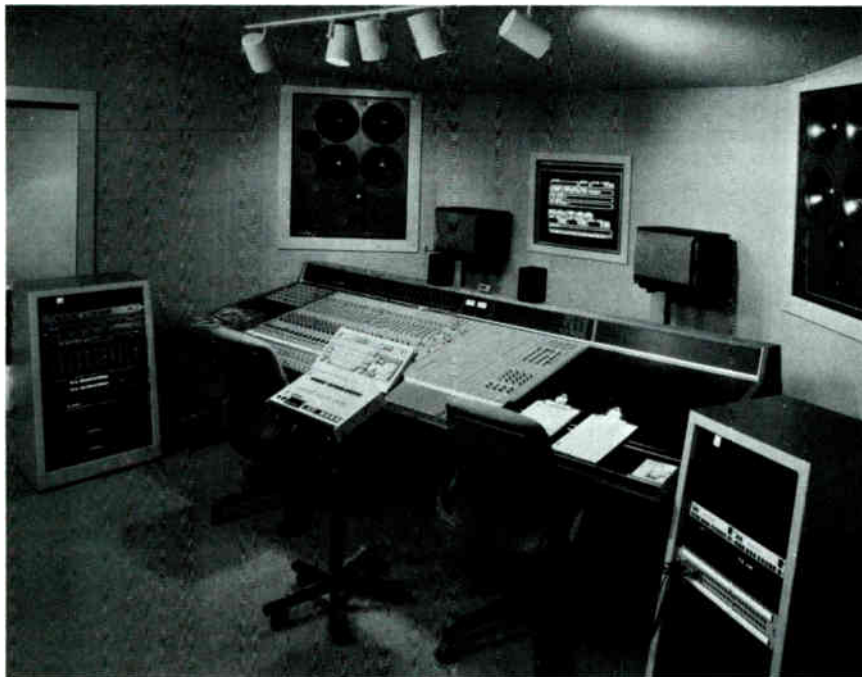
While it is state run, it's sure top flight—it's the new mixdown studio/classroom at Middle Tennessee State University. It features an extra-wide listening area and a Neotek Elite with moving faders.
