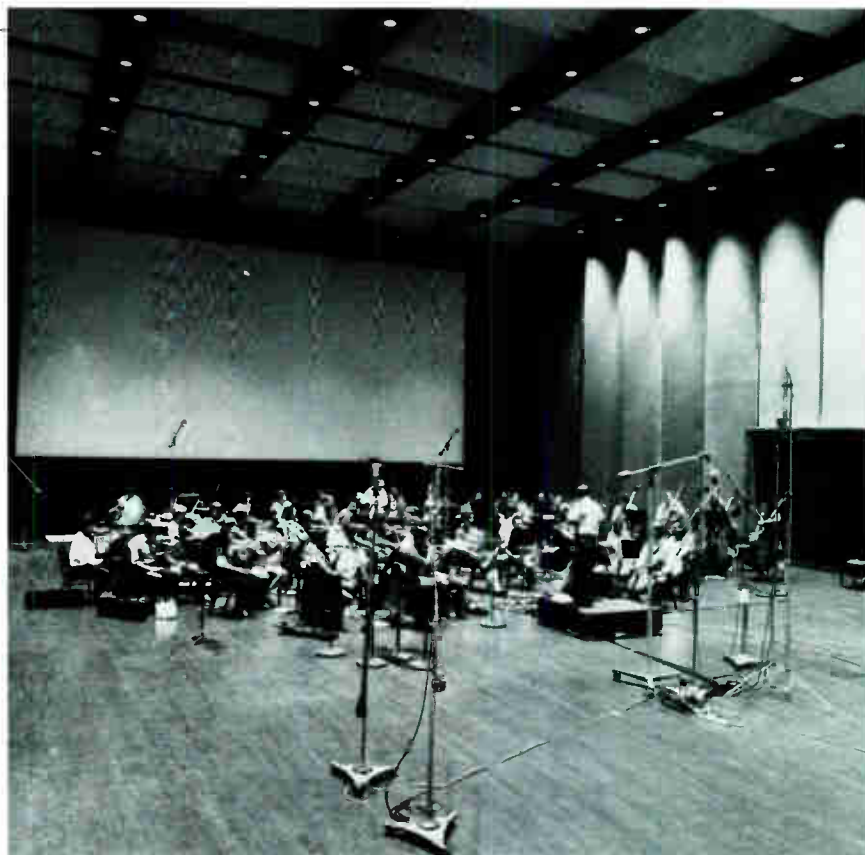
Members of the San Francisco Ballet Orchestra record the first session on the Skywalker sound stage. The 5,000 sq. ft. floor can accommodate up to 120 musicians; the viewing screen measures 48 x 38 feet. The walls and 29-foot ceiling have retractable baffles that can alter reverberation from .7 to 3.5 seconds. Jack Leahy and Gary Clayton from San Francisco's Russian Hill Recording engineered this session and tested the room's many sonic variables, completing post-production at their studio.
