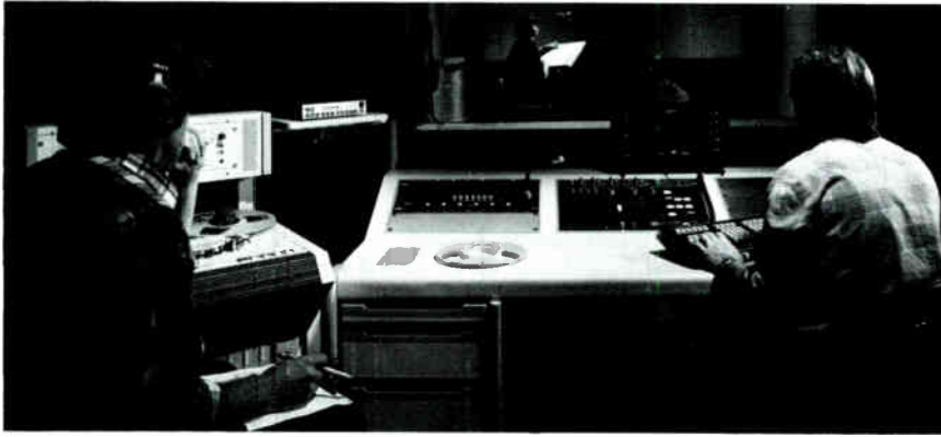
The ADR (Automated Dialog Replacement) stage uses an MTE ADR controller, 6-track 35 mm and 1-track 35 mm recorders with Dolby SR, and Otari 2- and 24-track machines with SR. Both 35 mm projection and video are available.
