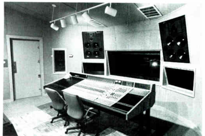
(R) The Welk Music Group's Nashville studio, a 1,895-sq.-ft. 24-track facility designed in 1985 by Bob Todrank, within a $375,000 budget. It contains four iso booths and a large control room. (L) Todrank implemented LEDE™ concepts and used RPG™ broadband and low frequency diffusors. The all-dome Boxer monitoring system was imported from London, installed along with the Neotek Elite console and Otari analog tape machines.
