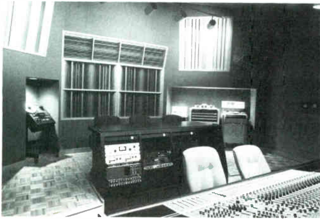
(R) The Welk Music Group's Nashville studio, a 1,895-sq.-ft. 24-track facility designed in 1985 by Bob Todrank, within a $375,000 budget. It contains four iso booths and a large control room. (L) Todrank implemented LEDE™ concepts and used RPG™ broadband and low frequency diffusors. The all-dome Boxer monitoring system was imported from London, installed along with the Neotek Elite console and Otari analog tape machines.
