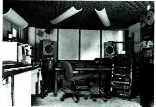
F. The new MIDI room at Synchro International Studios in San Anselmo, CA, features the TAC Scorpion console and Fostex E16 recorder with 4050 locator, and Sony PCM 601-ES digital recording processor. Keyboards include an Emulator II+HD, units by Roland, Yamaha, Oberheim and Korg, and the studio utilizes a Macintosh computer with Mark of the Unicorn software (with Opcode Interface) for sequencing. Designer was Daniel Ryman.
