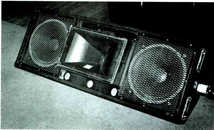
A Tecron TEF System 10 analyzer helped design MD Systems' JBL vocal monitors. Two E-140 woofers are coupled with a 2385 horn and 2445 driver.
