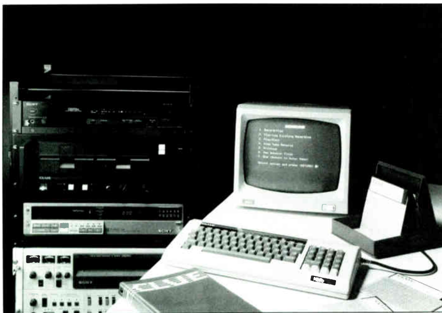
The CLUE logging/editing system is designed to work with tapes recorded in the Sony PCM-F1/701 digital format.
