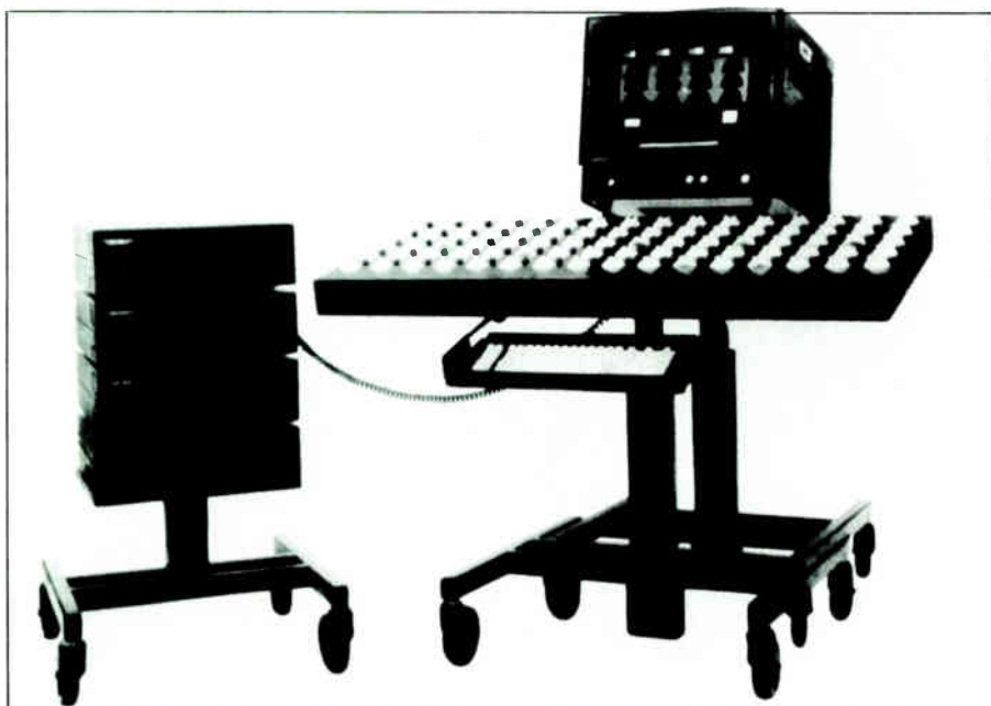
The CompuSonics DSP-2000, a disk-based audio recording/mixing/editing/retrieval system, is based on four-track digital storage modules.
