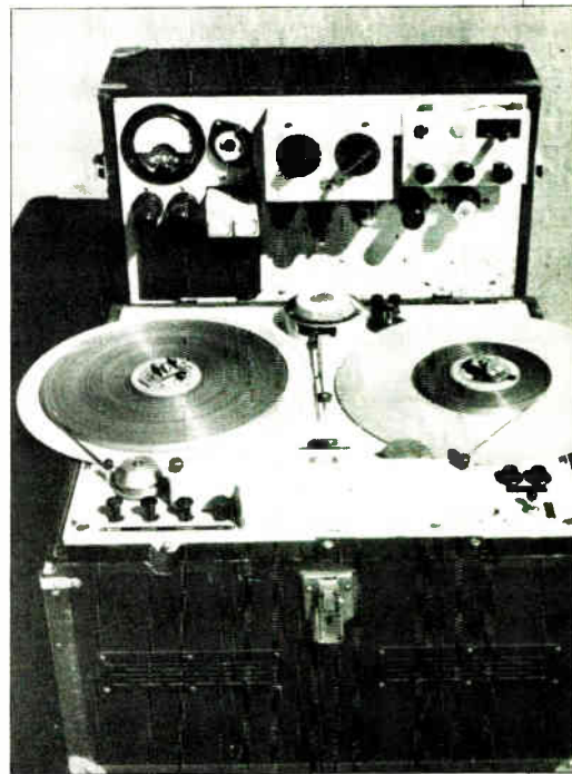
One of two Magnetophons employed by the author to record the Bing Crosby radio show in 1947. Electronics panel at rear was made up of American components following German circuits.
