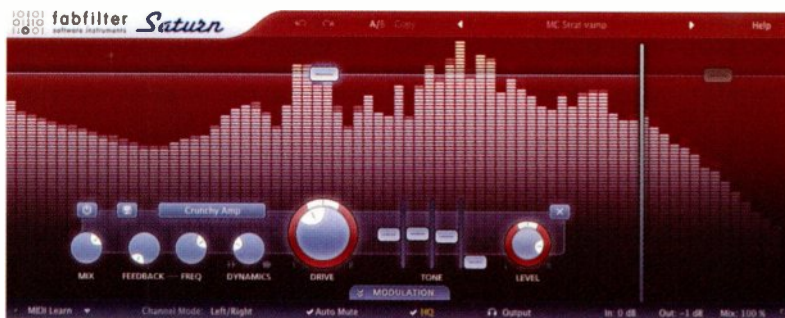
Figure 1: You can hide the modulation section of Saturn's GUI to streamline your workspace. The controls for band 1 (one of two frequency bands) are shown here.
