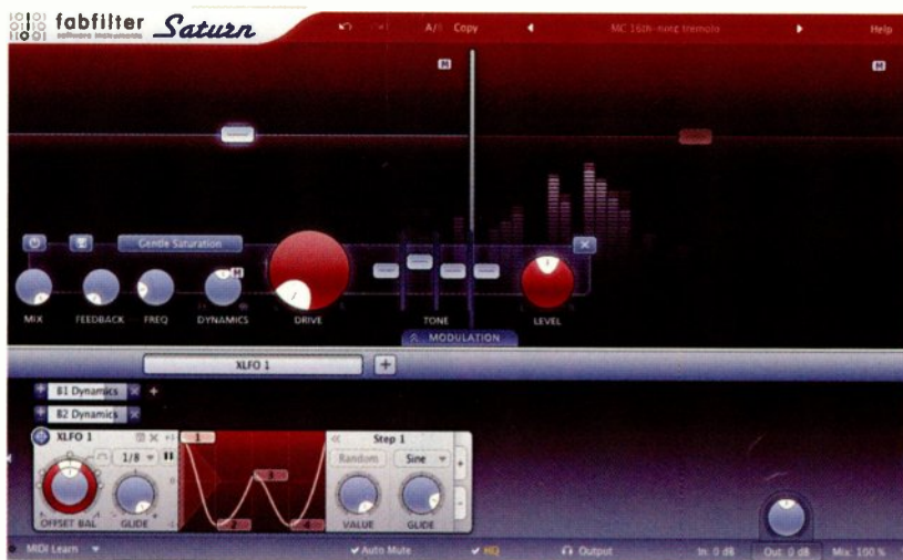
Figure 2: Saturn's GUI with the modulation section showing. An XLFO is modulating the dynamics controls for two bands to different degrees.
