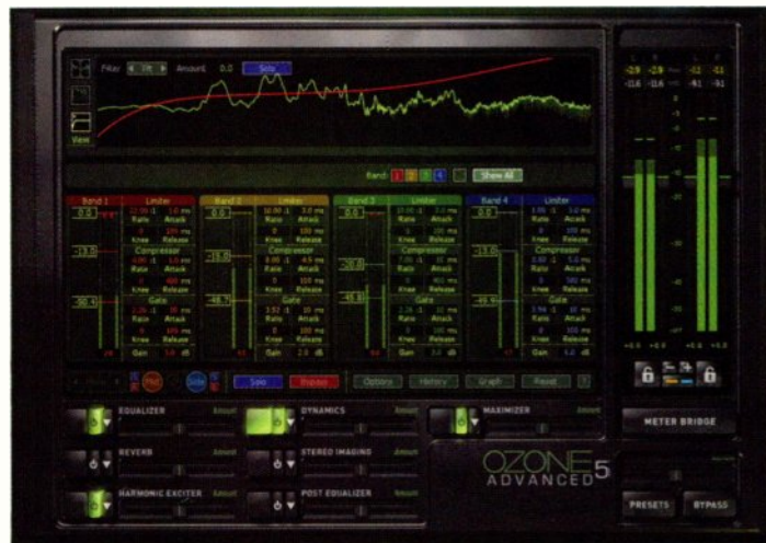
Fig. 1: The dynamics processor for Ozone 5 Advanced can now show the limiter, compressor and gate parameters for all frequency bands at once. The sidechain's Tilt filter is displayed at the top of the GUI.
