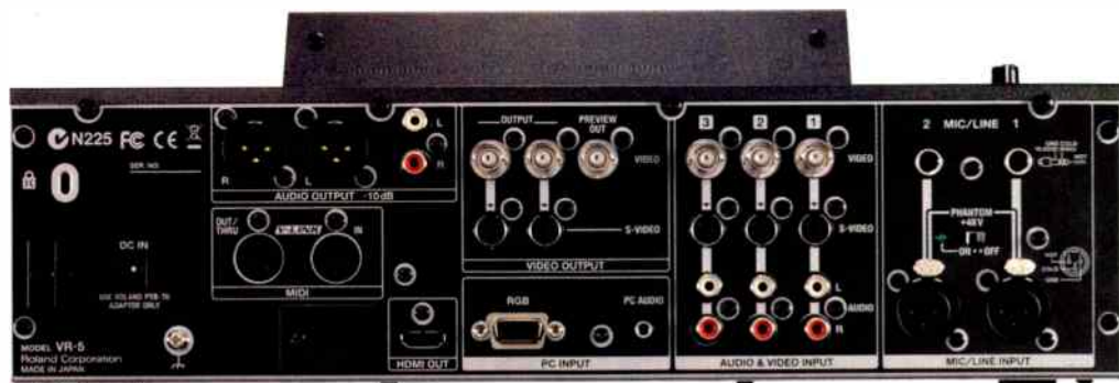
The back of the unit is packed with a variety of I/O and a V-Link connection to other Roland gear.
