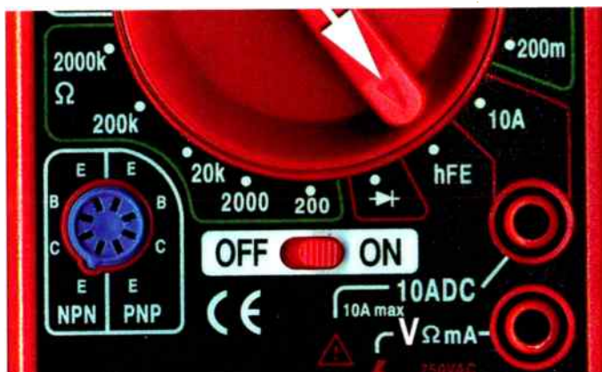
Figure 1: This multimeter tests diode and static transistor hFE.
