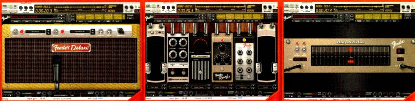
From left: You can move mics on- or off-axis, near or far, and add room ambience. The package also includes rack and stomp effects and a tuner.
