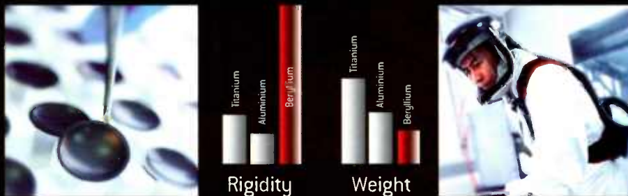
Comparison between Beryllium, Titanium and Aluminium. Beryllium is lighter and nearly five times more rigid.
