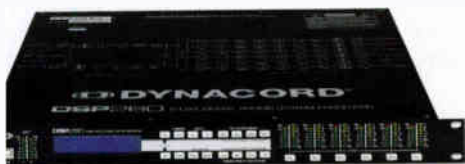
Dynacord DSP 260 24-bit system controller
