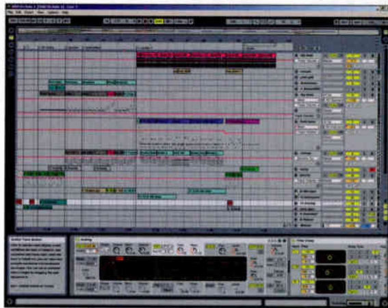
Tracks in Live's Arrangement view have their headers at the right. Automation envelopes (red lines) are displayed on top of the track data.
