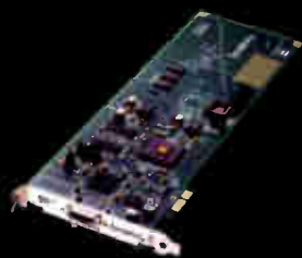
Symphony PCI Card 32 Channel, 192 kHz, 100 dB
