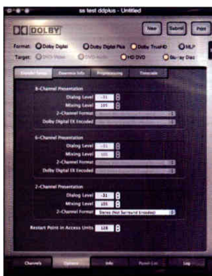
Dolby True HD encoder features 8-channel, 6-channel and downmix options for both HD-DVD and Blu-ray.
