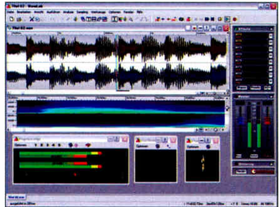
In Spectrum mode, users can identify and edit specific frequencies, leaving adjacent frequencies nearly untouched.
