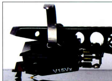
Figure C: The VTA (seen under stylus) is optimized when the arm and headshell are parallel to the disc surface. This is accomplished when the user raises or lowers the arm at the pivot point.
